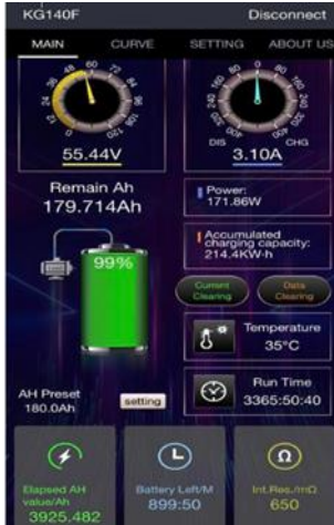
Scenario 1: Power Source: OFF, Inverter: ON, HVAC: OFF, Battery: Full
